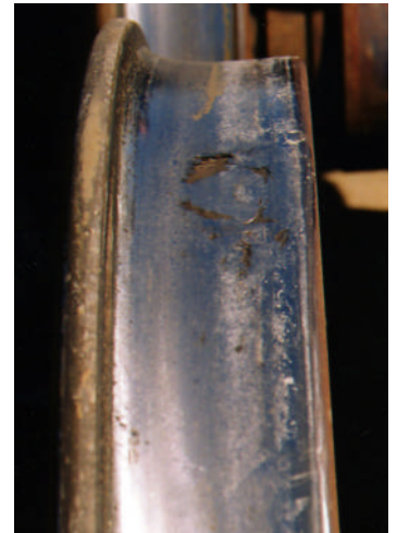
Photo of damaged wheel taken at the CSX repair shops.
