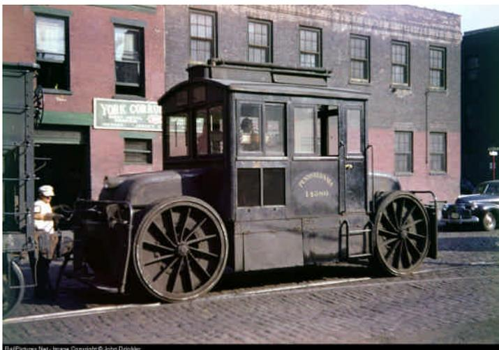
The Pennsylvania RR had a fleet of rubber tired switchers, first built 1912, originally battery powered & later repowered with gasoline engines. They worked the dockside industries in Philly, Baltimore, & Jersey City.
